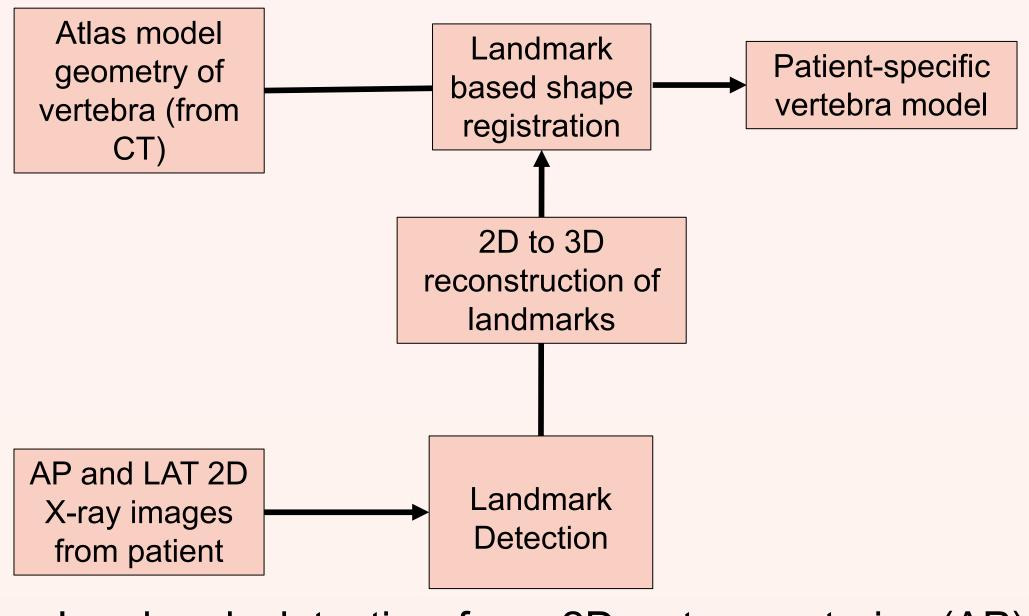
• Landmark detection from 2D anteroposterior (AP) and lateral (LAT) X-rays using novel B-spline based image segmentation:
