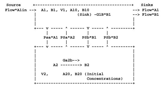
We next construct a model for two species with inflow of species A, exchange of A between two compartments, irreversible reaction converting A to Bin non-flowing compartment, exchange of B between the two compartments, consumption of B in the flowing compartment and outflow of A and B.
