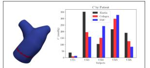
**Figure 1**: (a) The arterial model of the patient #1 (UM1), female 9 y/o, with larger main PA compared to right and left PA. (b) The initial stiffness of the PA for four patients and a healthy subject of the three vascular constituents, Elastin, Collagen and Smooth Muscle.
